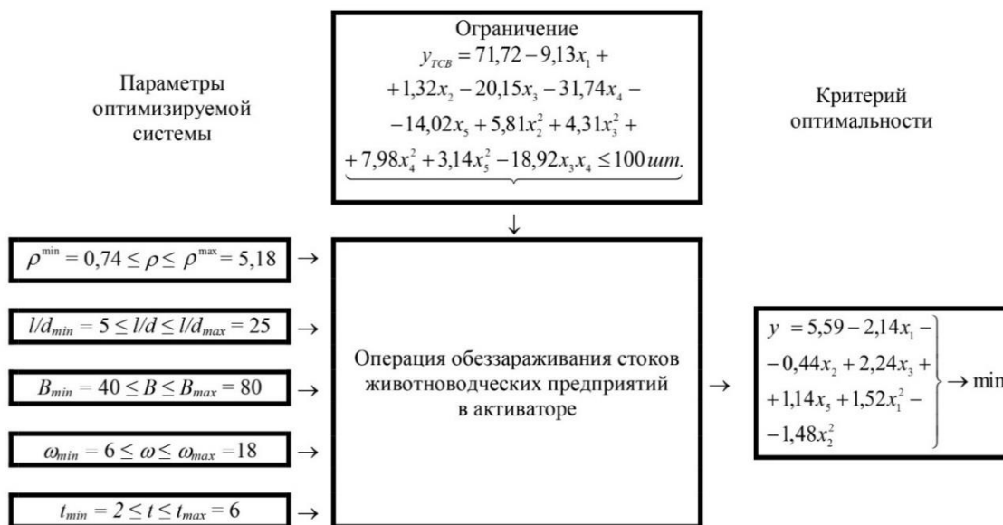
Fig. 2. The block diagram of the optimization problem
