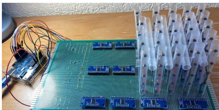
Figure 1 – Spatially distributed electromagnetic field sensor
